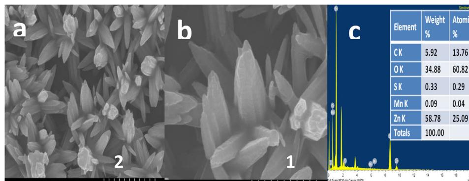
**Figure 2.** a-b) The SEM Images of ZnO NR at two magnifications. c) EDAX spectra.
