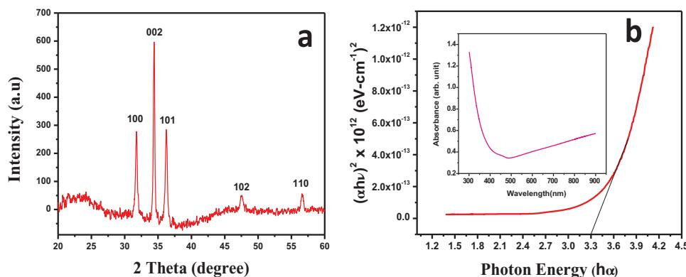
**Figure 1.** a) The X-ray diffraction pattern of ZnO NR. b) UV-Visible Spectra of Tauc's plot and absorption spectra (inset) for ZnO NR.
