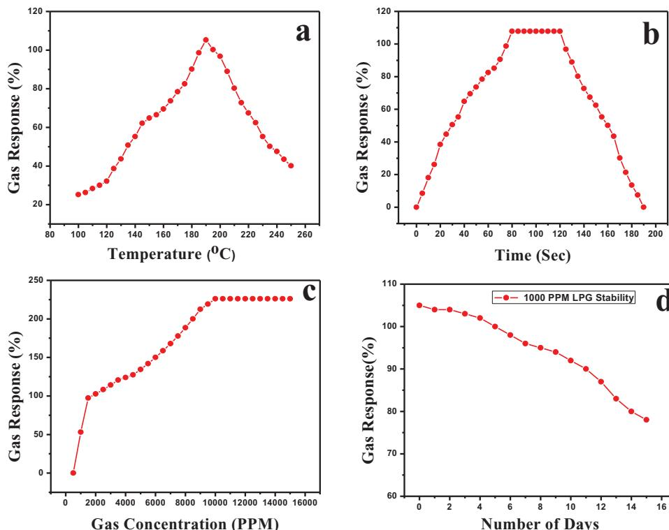
**Figure 3.** **a)** The variation of Gas response (%) with respect to operating temperature at 1000 ppm of LPG gas concentration. **b)** Response and Recovery plot at 190°C operating temperature. **c)** Variation of Gas response (%) with respect to LPG gas concentration. **d)** Long-term stability curve of ZnO NR for 100 ppm of LPG gas concentration.
